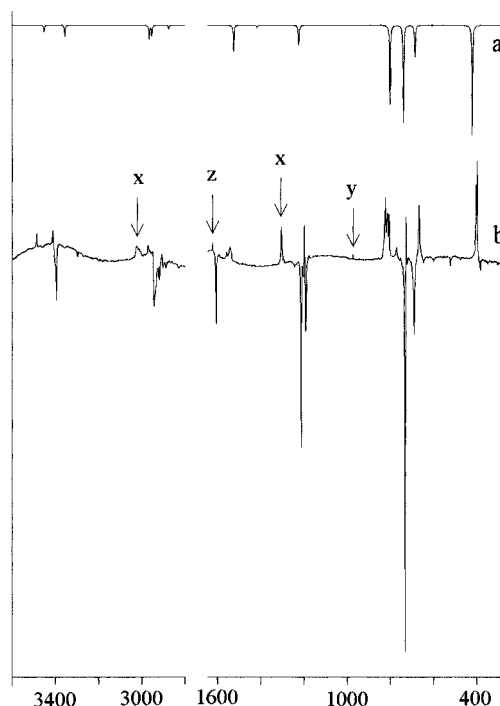
Figure 3. Irradiation of Me 3 Al·NH 3 in argon at 10 K: X-axis, 250–1650 and 2800–3600 cm -1 ; Y-axis, Absorbance (dimensionless). Spectrum a: Me 2 AlNH 2 calculated at the RMP2(fc)/6-31G* level (frequencies scaled by 0.93, half band width of 2 cm -1 ). Spectrum b: Difference IR spectrum after irradiation (210 nm) 13 of Me 3 Al·NH 3 for 7 h (decreasing absorptions point down, increasing absorptions point up). x indicates CH 4 (1304.0, 1306.5, 3024.0 (br) cm -1 ), y indicates NH 3 (974.5 cm -1 ), and z indicates H 2 O (1624.0 cm -1 ).
